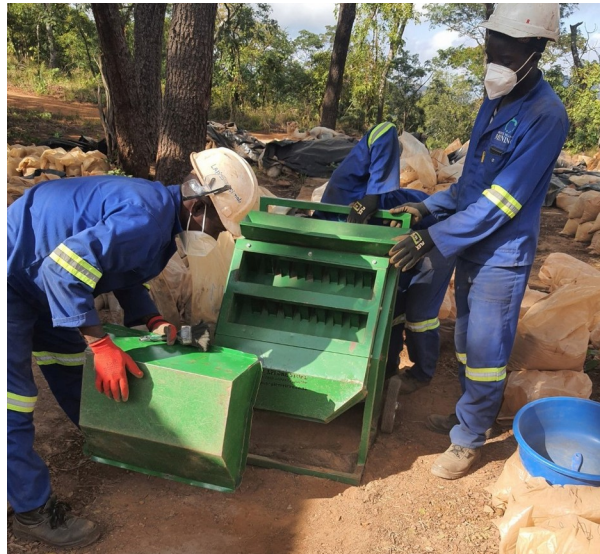
Figure 23: Riffle Splitting of RC samples in Progress by Altona Staff.
